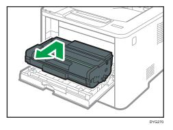
• Do not shake the removed print cartridge. Doing so can cause remaining toner to leak.
