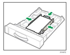
Check there are no gaps between the paper and the fences; both side and end fences.
