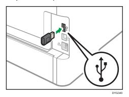
Check that the option is firmly connected to the USB port.
