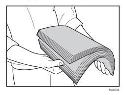
4. Load the paper in the tray with the print side faced down.
