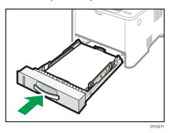
12. If paper is loaded in the bypass tray, remove the paper and close the bypass tray.
