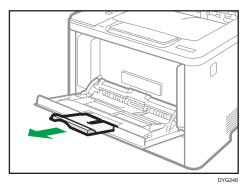
2. Slide the side fences outward, then load paper with the print side up, and push in until it stops against the machine.
