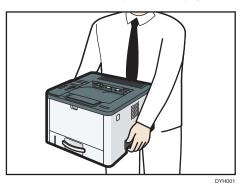
4. There are three upright pins on the optional paper feed unit. Align the holes of the machine with the pins, and then lower the machine slowly.
