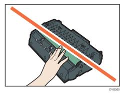
• Do not touch the ID chip on the top of the print cartridge as indicated in the illustration below.
