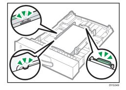
6. Carefully push the paper tray straight into the machine. To avoid paper jams, make sure the tray is securely inserted.
