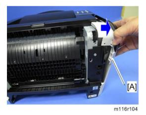
5. Pull the rear upper part [A] of the left cover to release the hooks.
