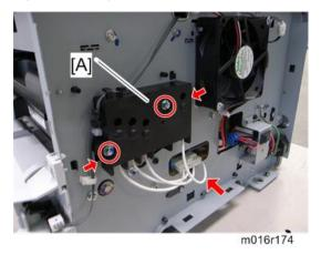
2. Charge terminal case [A] with the harness (🌮 x 2, 💷 x 1, hooks)
