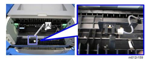
2. Relay sensor [A] (💷 x 1, hooks)
