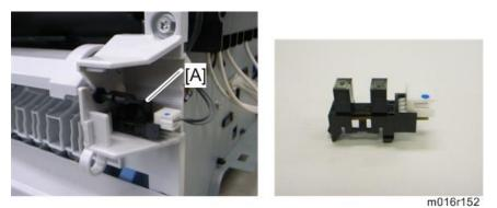
3. By-pass feed sensor [A] (hooks, 📬 x 1)
