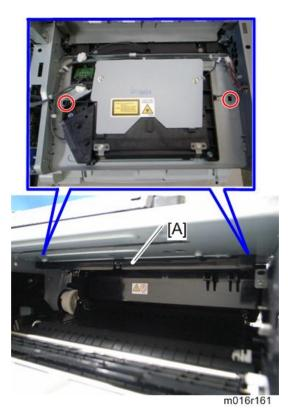
2. Release two hooks of the quenching lamp with the case [A], and remove it.
