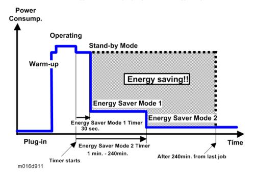
The backlight of the screen is turned off and "Energy Saver Mode 1" appears on the screen, and then the fusing lamp is turned off and "Energy Saver Mode2" appears on the screen.
