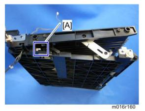
2. Inverter sensor [A] (💷 x 1, hooks)
