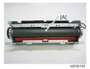
4. Hot roller [A] (C-ring x 2, gear x 1, bushing x 2)
