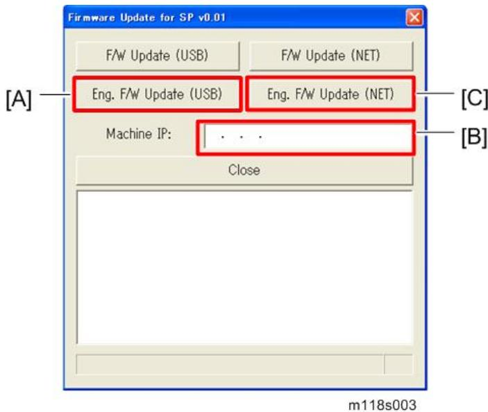
6. For a USB connection, click "Eng. F/W Update (USB)" [A]. For a network connection, enter the machine's IP address in "Machine IP" [B], and then click "Eng. F/W Update (NET)" [C].
