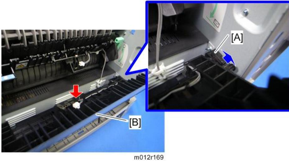
17. Release the lock [A], and then remove the entrance guide [B] (🔧 x 1).
