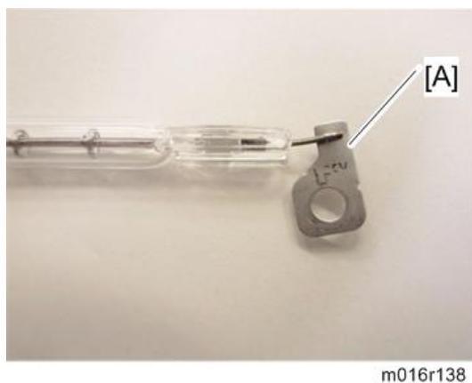
The flat terminal [A] must be placed on the right side of the fusing unit (fusing cable side).
