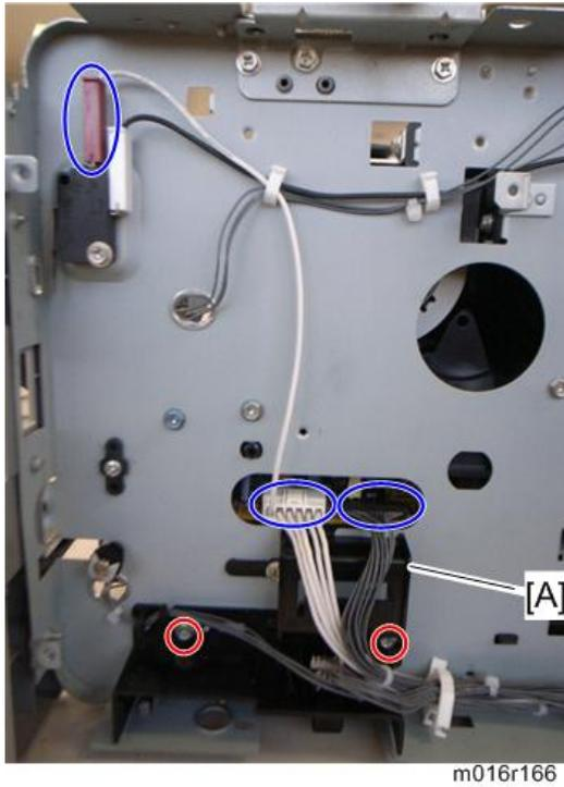
11. Disconnect three connectors in left frame (🔧 x 1)
