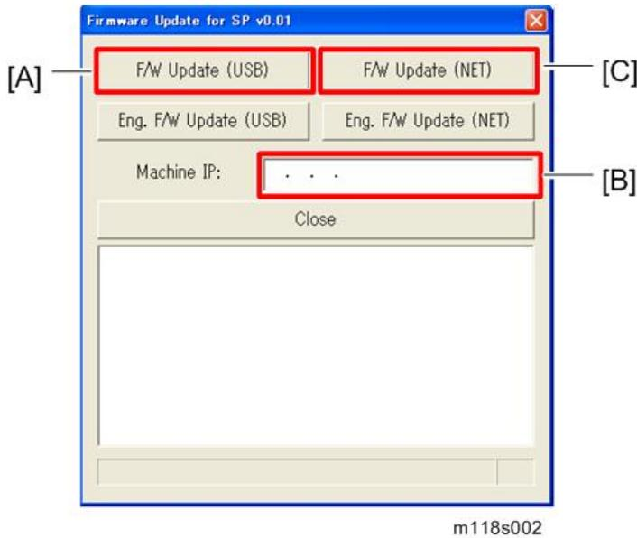
6. For a USB connection, click "F/W Update (USB)" [A]. For a network connection, enter the machine's IP address in "Machine IP" [B], and then click "F/W Update (NET)" [C].
