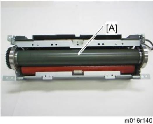
3. Hot roller [A] (C-ring x 2, gear x 1, bushing x 2)
