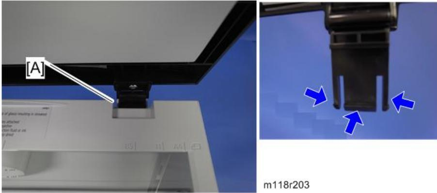
4. Release the three hooks of the right hinge [A].
