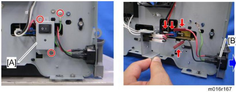
13. Main power switch bracket [A] in right frame (🔧 x 2)
