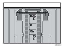
When loading custom size paper, position the paper guide slightly wider than the actual paper size.
