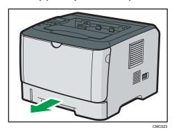
13. Remove the protective material attached inside the tray.
