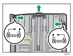
4. Lock the extender in the extended position.
