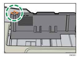
8. Check there are no gaps between the paper and the paper guides; both side and end paper guides.
