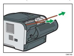
The actual printer may come with protective materials attached in different positions. Make sure to check the printer's exterior for all protective materials, and remove them completely.
