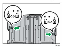
5. Pinch the clip on the side paper guide, and then slide it to match the standard size.
