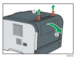
5. Pull out the tape, and then remove the protective materials.
