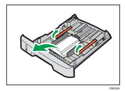
14. Carefully push tray 1 straight into the printer.
