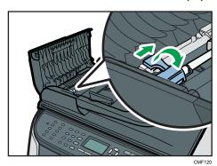
4. Lift the paper feed roller slightly and pull it out toward you.
