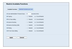
5. Under "Available Functions", enter the timeout value in seconds (5 to 60, the default is 30) in [User Authentication Timeout (Copy)].
