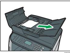
6. If you cannot pull out the jammed original easily, raise the input tray to see if the original is jammed in the output area.
