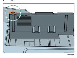
Check there are no gaps between the paper and the paper guide; both side and end paper guides.
