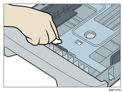
Wipe the rubber part of the roller with a soft damp cloth. After that, wipe it with a dry cloth to remove the moisture.
