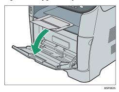
2 Slide the side guides outward, then load envelopes with the print side up, and push in until it stops against the machine.
