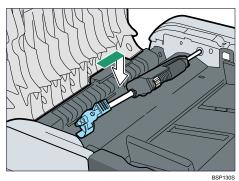
2 Lower the blue lever to lock the paper feed roller.
