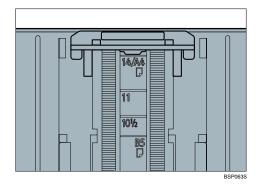
When loading custom size paper, position the paper guide slightly wider than the actual paper size.
