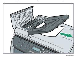
1 Put the paper feed roller back in with the roller part facing downwards.
