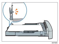
If there is a gap between the paper and the end paper guide, as in the example below, the paper might not feed in correctly.
