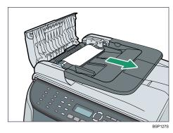
If you cannot pull out the jammed original easily, raise the input tray to see if the original is jammed in the output area.
