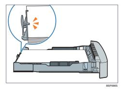
6 Slide the tray, then push it all the way in. Push the tray firmly to avoid a paper jam.
