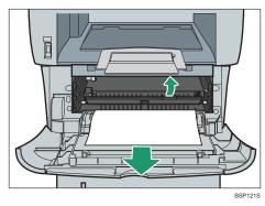
Slide the print cartridge in horizontally. When the cartridge can go no further, raise it slightly and push it fully in. Then push down on the cartridge until it clicks into place.
