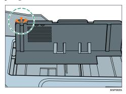
Check there are no gaps between the paper and the paper guides; both side and end paper guides.
