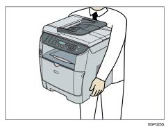
There are three upright pins on the optional paper feed unit. Align them with the holes on the underside of the machine, and then carefully lower the machine onto them.
