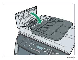
Lift the ADF, and if there is original remaining in the ADF, gently pull the jammed original to remove it.
