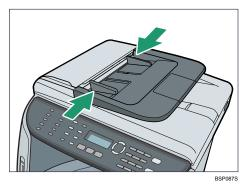
2 Place the aligned originals face up in the ADF. The last page should be on the bottom.
