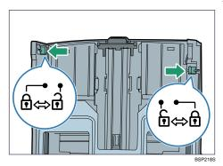
Pinch the clip on the side paper guide, and then slide it to match the standard size.
