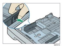
Pinch the clip on the end paper guide and slide it inward to match the paper size.
