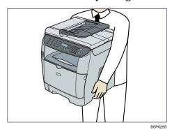
**3** Remove the protective materials attached on the machine's exterior.
