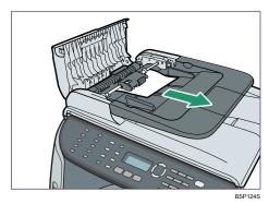
If you cannot pull out the jammed original easily, move the blue lever slightly to the machine rear, and then raise it to unlock the paper feed roller.
