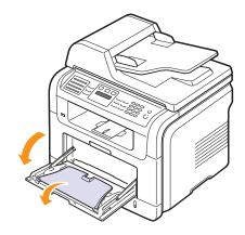
If you are using paper, flex or fan the edge of the paper stack to separate the pages before loading.
