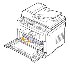
Thoroughly roll the cartridge 5 or 6 times to distribute the toner evenly inside the cartridge.
