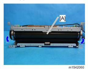
12. Remove the C-ring x 2, gear x 1, cap x 1, bushing x 2 from the Hot Roller.
