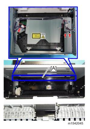
5. Remove the quenching lamp [A] from the case (hook  $\times$  3).
