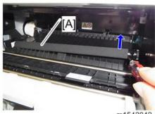
4. Remove the bushing x 2, spring x 2, gear x 1, collar x 1 from the transfer roller.
