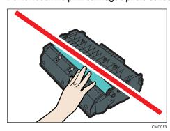
Do not touch the ID chip on the side of the print cartridge as indicated in the illustration below.
