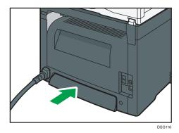
3. Release the extender lock on the left rear of the tray, and then pull out the extender until it clicks.
