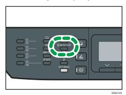
Press the [♠], [♥], [◄], or [▶] key to select the desired resolution, and then press the [OK] key.
