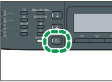
2. Press the One Touch button to which the desired Quick Dial entry is registered.
