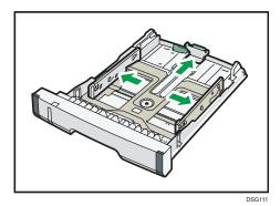
3. Fan the paper and load it in the tray with the print side faced down.
