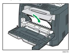
14. Slide the print cartridge in horizontally. When the cartridge can go no further, raise it slightly and push it fully in. Then push down on the cartridge until it clicks into place.
