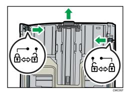
4. Lock the extender in the extended position.
