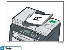
• When placing originals longer than A4, pull out the ADF tray's extenders.
