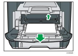
12. Lifting the guide plate, remove the jammed paper carefully.
