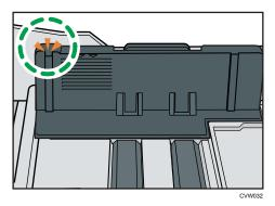
5. Check there are no gaps between the paper and the paper guides; both side and end paper guides.
