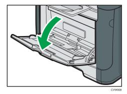
2. Slide the side guides outward, then load envelopes with the print side up, and push in until it stops against the machine.
