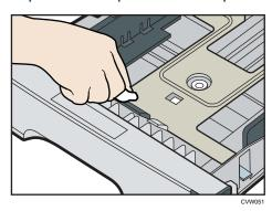
5. Wipe the rubber part of the roller with a soft damp cloth. After that, wipe it with a dry cloth to remove the moisture.
