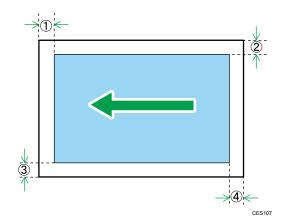
Margins when using exposure glass
