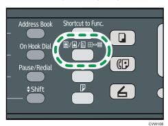
2. Press the [♠], [♥], (◄], or [▶] key to select the desired resolution, and then press the [OK] key.
