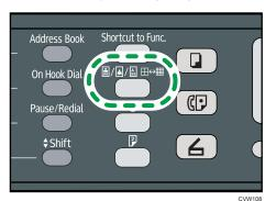
Press the [▲] or [▼] key to select the desired resolution setting, and then press the [OK] key.
