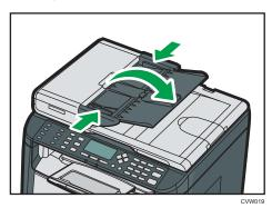
2. Place the aligned originals face up in the ADF. The last page should be on the bottom.
