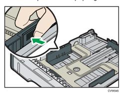
When loading custom size paper, position the paper guide slightly wider than the actual paper size.
