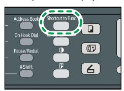
To make the [Shortcut to Func.] key enable ID card copy mode for the current job, [Shortcut to Function] under administrator settings must be set to [ID Card Copy Mode].
