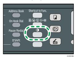
2. Press the [▲] or [▼] key to select the desired density level, and then press the [OK] key.
