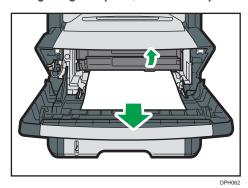
8. Slide the print cartridge in horizontally. When the cartridge can go no further, raise it slightly and push it fully in. Then push down on the cartridge until it clicks into place.
