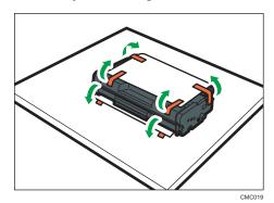
6. Hold the print cartridge and shake it from side to side five or six times.
