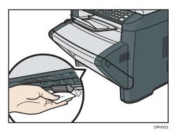
6. Reload the removed paper into the tray, and then push the tray carefully into the machine until it clicks into place.
