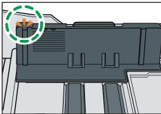
5. Check there are no gaps between the paper and the paper guides; both side and end paper guides.
