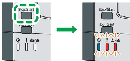
The Power indicator, Alert indicator, and Toner/Paper End indicator will repeatedly flash in this order, and the machine starts to connect in PBC method.
