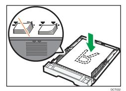
6. Check there are no gaps between the paper and the paper guides (both side and end paper guides).
