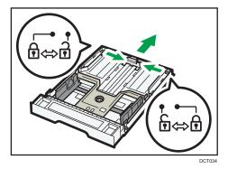
Make sure the extender's inner surface and the scale are aligned.
