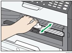
Wipe carefully so as not to touch any protrusions inside the machine.
