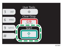
5. Within 60 seconds, place the original back side down with the upper-left corner on the exposure glass, and then press the [Start] key.
