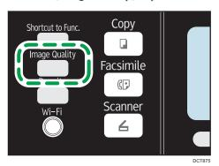
Press the [♠], [♥], (♥], or [▶] key to select the desired document type, and then press the [OK] key.
