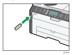
"Loading..." appears on the display. Wait until the display changes to show "Save Scn Data to USB" (the duration depends on your USB flash disk).
