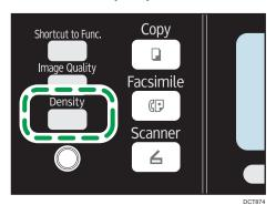
2. Press the  $[^{\blacktriangle}]$  or  $[^{\blacktriangledown}]$  key to select the desired density level, and then press the [OK] key.
