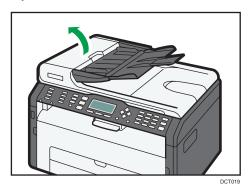
2. Gently pull the jammed original to remove it. Be careful not to pull the original too hard, as it may tear.
