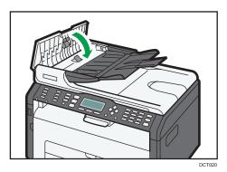
4. Lift the ADF, and if there is original remaining in the ADF, gently pull the jammed original to remove it.
