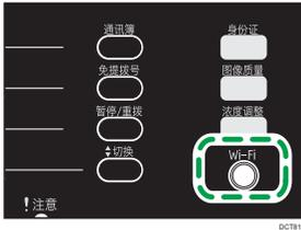
If [Wi-Fi Enable] is set to [Disable], you cannot use the [Wi-Fi] key. If [Frequency Channel] appears first, set [Wi-Fi Key] to [Infrastructure Mode].
