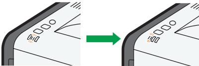
The alert indicators start flashing, then, after 30 seconds, the alert indicator goes out and the power indicator lights continuously.
