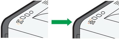
The alert indicators start flashing, then, after 30 seconds, the alert indicator goes out and the power indicator lights continuously. Also, the [Wi-Fi] key stops flashing.
