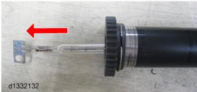
4. Lay the fusing lamp on a clean flat surface.
