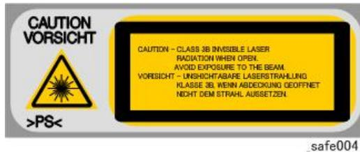
1. The Center for Devices and Radiological Health (CDRH) prohibits the repair of laser-based optical units in the field.
