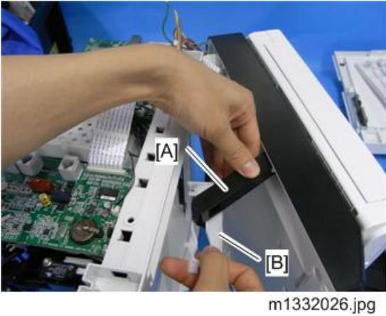
7. Bend and release the joint part with a screwdriver to detach the hinge.
