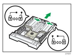
Make sure the extender's inner surface and the scale are aligned.
