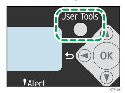
Press the [▼] or [▲] key to select [System Settings], and then press the [OK] key.
