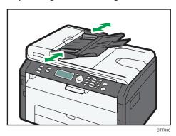
3. Place the aligned originals face up in the ADF. The last page should be on the bottom.
