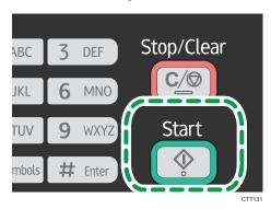
When you place the original on the exposure glass, perform the following steps to scan the subsequent pages of the original.
