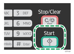
6. Within 30 seconds, place the original back side down with the top to the rear of the machine on the exposure glass, and then press the [Start] key.
