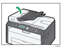
2. Gently pull the jammed original to remove it. Be careful not to pull the original too hard, as it may tear.
