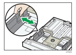
3. Pinch the end paper guide and slide it inward to match the standard size.
