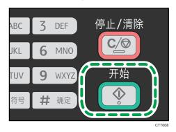
6. Within 30 seconds, place the original back side down with the top to the rear of the machine on the exposure glass, and then press the [开始] key.
