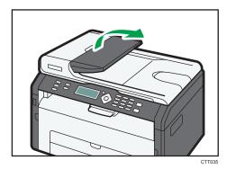
2. Adjust the guides according to the size of the originals.
