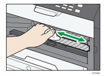
4. Slide the print cartridge in horizontally, and then slowly push it in all the way. Finally, push the cartridge down until it clicks into place.
