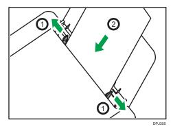
3. Do not load too much paper at a time. The feed tray can hold 50 sheets (A4 70g/m<sup>2</sup>) maximum.
