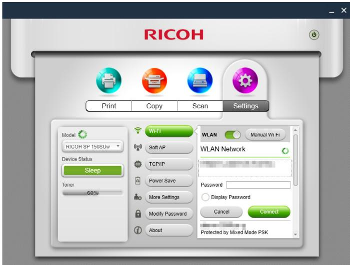
Toggle the WLAN switch to turn on or turn off Wi-Fi. The printer must be restarted for any change in Wi-Fi status to take effect.
