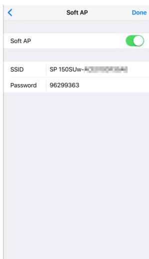
3. If the Soft AP function is turned on, enter the Service Set Identifier (SSID) and password for the Soft AP network. Tap [Done] to save the setting.
