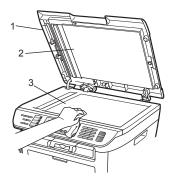
In the ADF unit, clean the white bar (1) and the scanner glass strip (2) underneath it with a soft lint-free cloth moistened with water.
