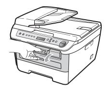
2 Slowly take out the drum unit and toner cartridge assembly. The jammed paper will be pulled out with the toner cartridge and drum unit assembly.
