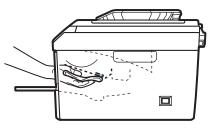
4 Put the drum unit and toner cartridge assembly back in the machine.
