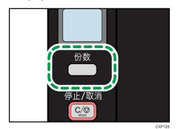
Holding down the [份数] key increases the number in increments of 10.
