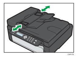
3. Place the aligned originals face up in the ADF. The last page should be on the bottom.
