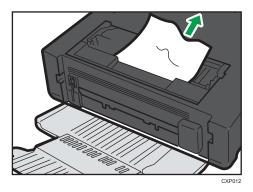
6. If it is difficult to remove the jammed paper out of the main unit, remove the jammed paper from the output tray side.
