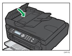
4. Lift the ADF, and if there is original remaining in the ADF, gently pull the jammed original to remove it.
