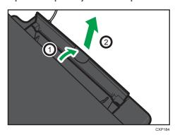
2. After pulling out the tray, tilt it back and forth, and then attach the end of the input tray to the machine.
