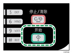
6. Within 30 seconds, place the original back side down with the top to the rear of the machine on the exposure glass, and then press the [开始] key.
