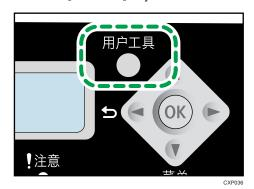
2. Press the  $[\,^{\blacktriangledown}]$  or  $[\,^{\blacktriangle}]$  key to select [System Settings], and then press the [OK] key.
