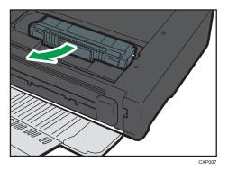
4. Push the Fusing Pressure Release Lever on the left down with your thumbs.
