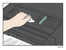
Wipe carefully so as not to touch any protrusions inside the machine.
