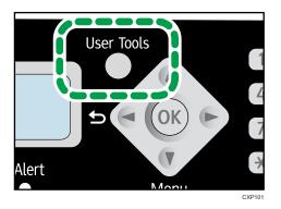
2. Press the [♥] or [▲] key to select [System Settings], and then press the [OK] key.
