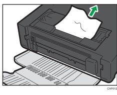
6. If it is difficult to remove the jammed paper out of the main unit, remove the jammed paper from the output tray side.
