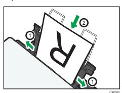
6. Adjust the paper guide on both sides to fit the paper width.
