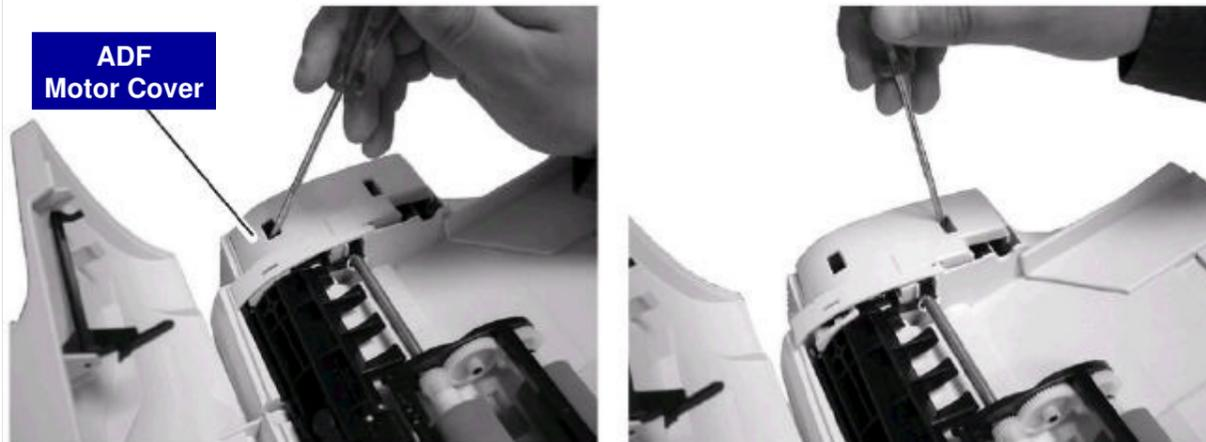
**Remove the ADF motor cover from its two slots using a flat screwdriver.**
