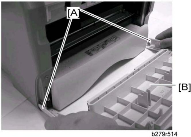
2. Push the left and right sides [A] of the front door and simultaneously pull it towards yourself.
