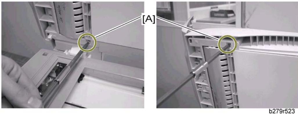
1. Lift the ADF cover and unscrew the two mounting screws [A] of the inside paper path assembly.
