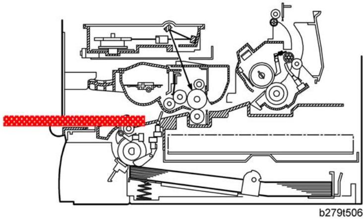
When the registration sensor does not turn on within 1.6 seconds after the main motor starts.
