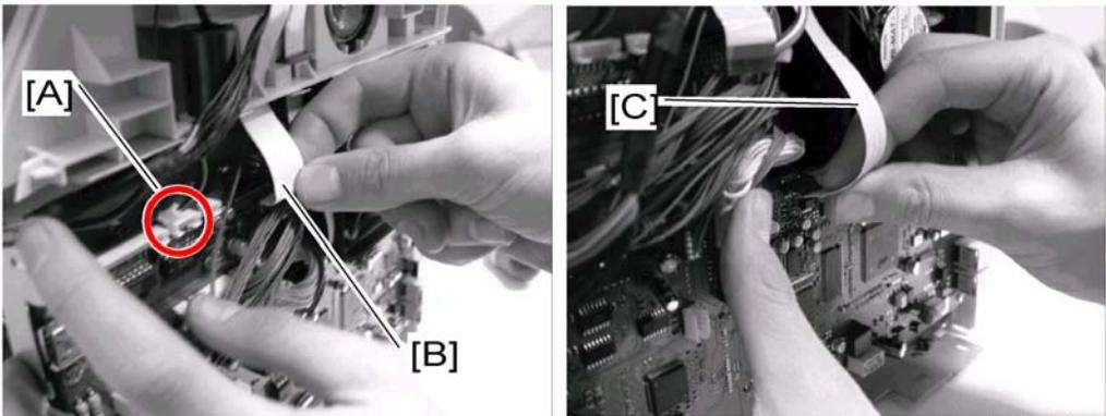
4. Disconnect the scanner connector [A] from the CPU board and remove it from its ferrite tube and cable guide.
