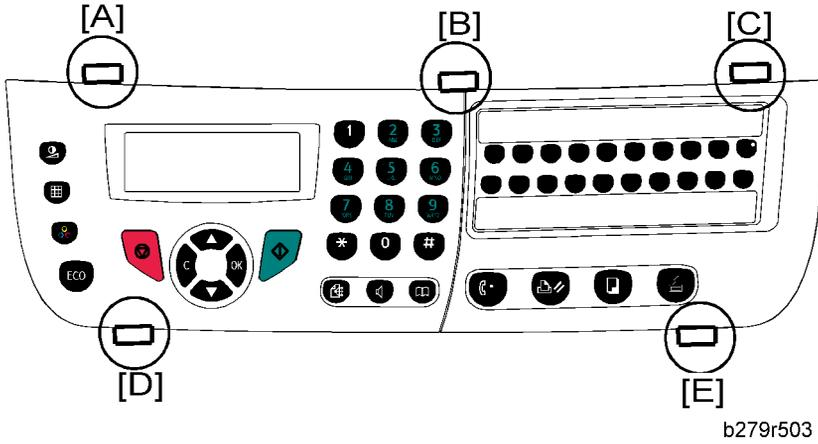
2. Unlock the three clips of the operation panel ([A], [B] and [C]).
