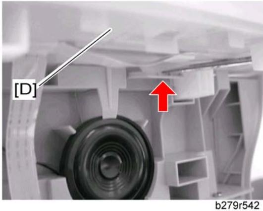
7. Unlock the assembled flatbed scanner [D] with a flat screwdriver and pull it towards yourself.
