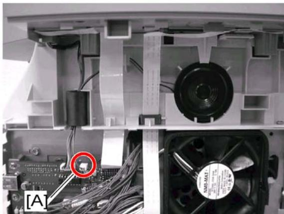
3. Disconnect the speaker connector [A] from the CPU board.
