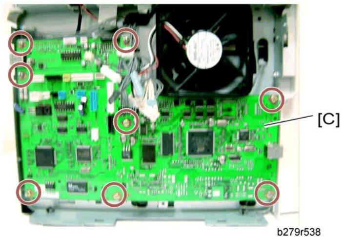
6. Unscrew the eight mounting screws and remove the CPU board [C].
