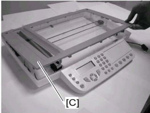
7. Lift the front part of the scanner frame [C] and remove it.
