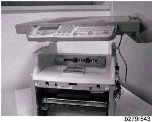
8. Lift the assembled flatbed scanner and remove it.
