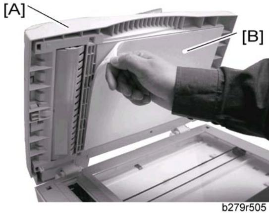
1. Stand in front of the machine and open the ADF scanner cover [A].
