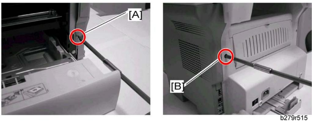
2. Unscrew the two mounting screws on the front [A] and back [B] of the side covers (right and left).
