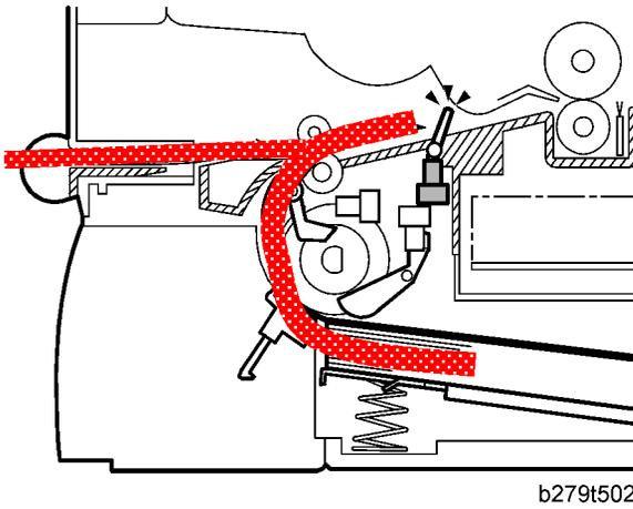
When the registration sensor does not turn on within 2.65 seconds after the paper pick-up clutch for the paper cassette turns on.
