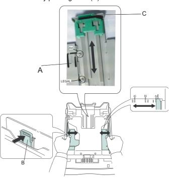
Take a paper stack, pull the paper off and align it on a flat surface.
