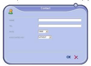
4 Enter the contact name as well as the fax number, the fax transmission rate with this person and the associated quick dial button. Click on OK.
