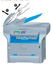
2 Remove the jammed paper without tearing it. The following message appears:
