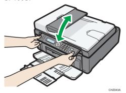
The machine will then slowly eject the jammed paper. After the jammed paper is ejected, remove it.
