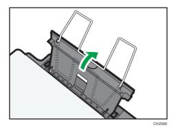
When closing the input tray, make sure to return the paper support wire to the correct location.
