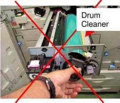
If the drum knob is loosened while the drum cleaner is installed, make sure to remove the drum cleaner before fastening the drum knob.
