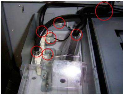
diag. 6-5. Attaching Connector and Tube
