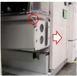
diag. 4-7. Removing the Oil Tank
