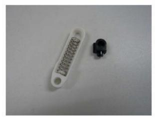
2-3 Removal of the silencer Remove the silencer at the tip of the shaft of the paper ejection guide board
