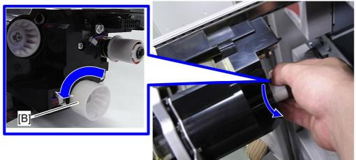
2. Turn the coupling gear [B] on the rear side of the development unit counterclockwise ten rotations or more as shown above. (This agitates the developer in the development unit, and then the developer becomes evenly distributed.)
