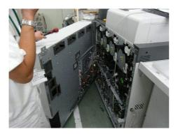
3. Remove the tube attached to the sub-hopper
