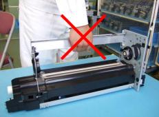
Applying external pressure will deform the front and rear plates in vertical and horizontal directions, resulting in fluctuation of the PG.
