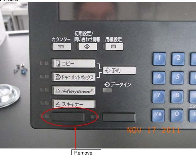
1. Remove the blank key top on the operation panel
