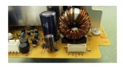
The wires break easily, so pull them from the board at the root of wires.
