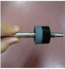
3-2-2 Removal and replacement of center rollers Remove the end rollers and the E-rings from the shaft. Again, be careful not to drop the balance pins.
