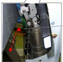
Remove the Exit Rollers by pulling it out horizontally, and then vertically.
