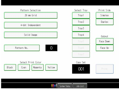
7. The configuration screen of the "Test Print Tool" automatically appears on the operation panel as shown above.
