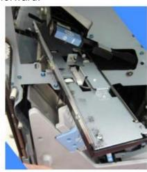
3 Removal of drive rollers Remove the guide board: paper ejection drive rollers
