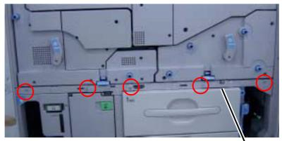
(2) Remove 3 mounting screws on the Bottom Cover of the Fusing Paper Exit Unit. [diag. 3-2.]
