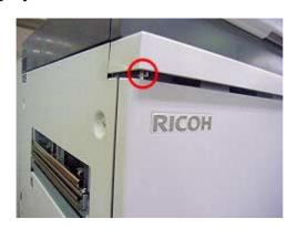
(2) Remove the front-left door inner Supporting Board (screw x11), Bracket: Door Catch (metal plate x2, screw x2), Lever-Safety Switch (molded part x1, screw x1) from the front-left door. [diag. 2]
