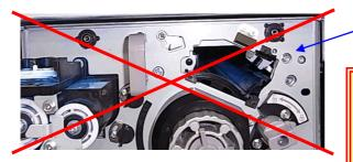
Never operate the machine without the Inner Cover or the screws.
