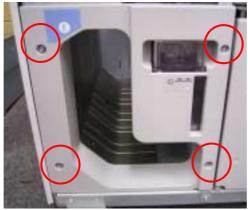
diag. 4-2. Removing the Oil Tank Front Cover
