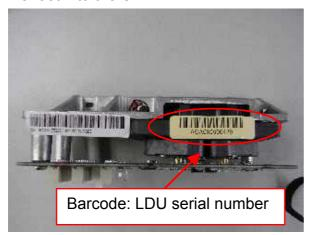
The barcode attached to the top-right of the LDU corresponds to the 11-digit LDU serial number indicated on the top-left of the data sheet.
