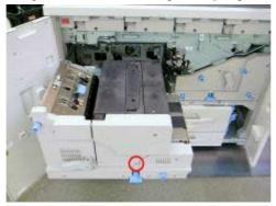
diag. 1-4. Mounting Screw on Fusing Unit
