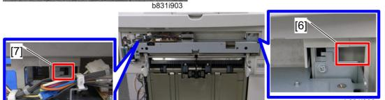
4. Align the hooks [4] [5] of the fan unit frame with the cutouts [6] [7] at the front and rear of the finisher frame.
