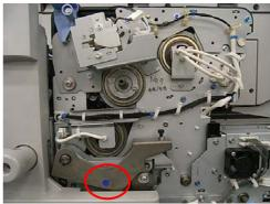
Although the units can be distinguished by the p/n indicated on the packaging boxes, it could be tricky after the units are installed in the mainframe. To enable distinction, the modified units are marked with blue stickers on the cover and the arm as shown in the photos above.
