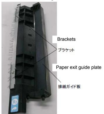
5. Attach "B3011216" (discharge brush for individual support) as shown in the photo below, then fasten it with the bracket to the paper exit guide plate.
