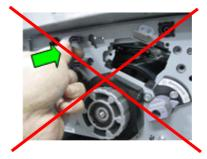
When the gears are not engaged properly, the drum cleaning unit pushes the drum towards the direction in which the PG is narrowed. Printing in this condition will cause toner to adhere to the development rollers and generate scratches on the drum surface.
