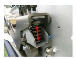
The pressure spring in the modified fusing unit has a marking along the side.
