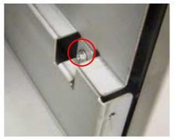
diag. 6-2. Assembling the new Upper Oil Tank Stand
