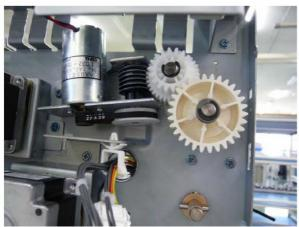
Then, remove the gear connected to the belt shaft. Please be careful not to drop the balance pin when removing the large lower gear. Remove the Sintering Bearing from the sideboard and remove the balance pin by pushing it through, it is difficult to remove.
