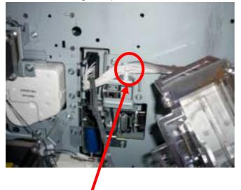
\* harness clamp located right below the motor holder
