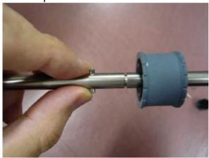
Square up the balancing pin with the new roller and slide it on. Be careful of the direction the roller is placed on the shaft, and then return the E-rings.
