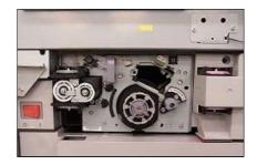
3. Remove the rear upper cover, and open the rear unit.
