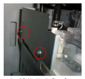
diag. 6-7. Attaching the Pump Cover
