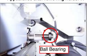
After removing the Holder-A, the ball bearing will remain and be of no use.
