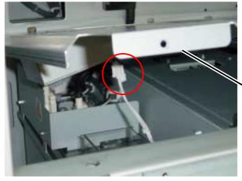
diag. 3-3. Disconnecting the Fan Connector
