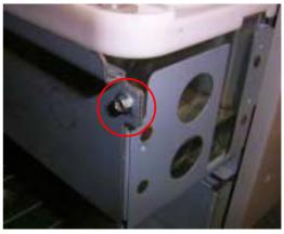
diag. 6-3. Assembling the Filtered Oil Tank
