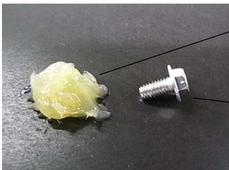
**1g of grease (1 cubic cm)****(Size reference) M4x8 screw**
