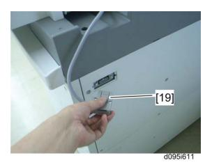
29. Connect the I/F cable [19] of the ADF to the LCT-MF.
