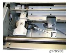
7. Rotate the shift roller unit motor [F] (it is actually under the shift roller unit) to move the shift roller unit [G] to the front side as far as possible.
