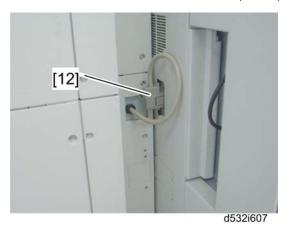
18. Attach I/F connectors [12] to the mainframe.
