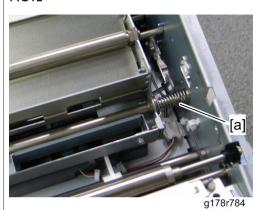
• When the shift roller unit shaft is pulled out, the spring [a] may spring out. Hold the spring [a] with your hand when you pull out this shaft.
