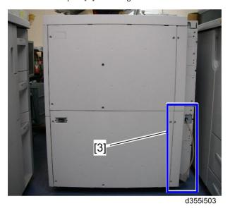
4. Remove the lower rear left cover [3] of the LCT (  $\rlap/F$  x 5)
