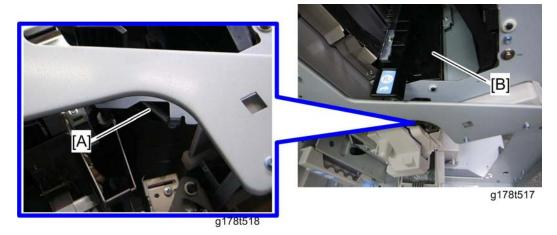
5. Remove the front tension spring [A] of the paper exit guide plate [B].
