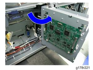
4. Open out the IOB 2 bracket fully.
