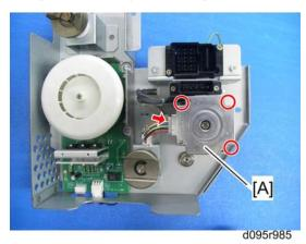
2. Pressure roller lift motor [A] ( 🎤 x 3, 🗂 x 1)
