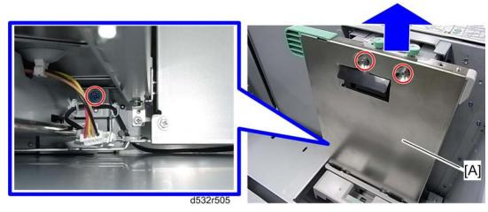
7. Pull up the front side fence [A], and then remove it (  $\slash\hspace{-0.4em}P \times 3$  ).
