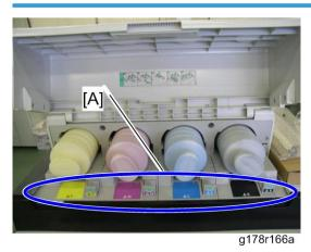
The area [A] shown above must be cleaned at 400 K intervals. Clean the area with a dry cloth.
