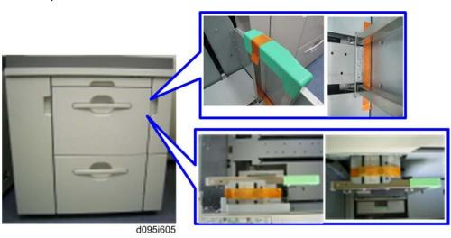
2. Remove all tapes in the upper and lower trays of the LCT-MF.
