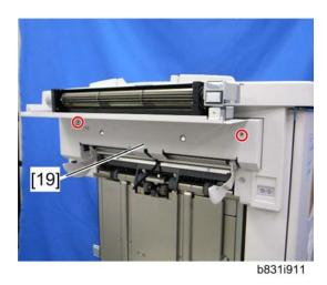
11. Install the lower cover [19] under the cooling fan unit (  $\rat{p} \times 2$  ).
