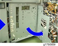
5. Unlock six clamps and disconnect all connectors.
