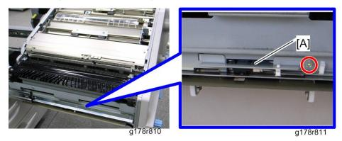
2. Duplex transport sensor 3 bracket [A] ( 🌶 x 1, 🖨 x 2, 📬 x 1)
