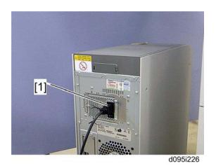
2. Connect the power cable [1] to the power cord socket on the rear side of the controller.
