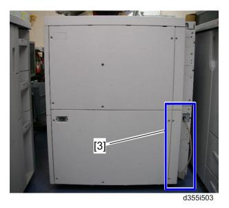
7. Remove the lower rear left cover [3] of the LCT-MF (  $\rat{F}$  x 5)
