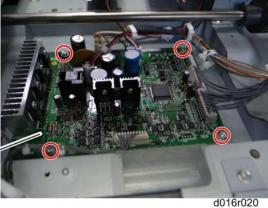
• Insert a screwdriver into the four holes (marked with arrows) on the bracket to remove the MCU board.
