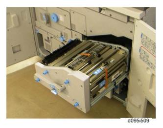
14. Remove all strips of tape, tags, and retainers from the registration unit.
