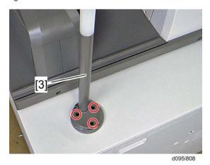
2. Stand the attention light [3] on the top of the controller box, and then fasten the attention light ( \*x 3; M3x8).
