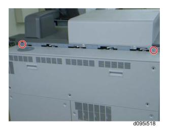
2. Remove the two screws attaching the rear controller box to the mainframe.
