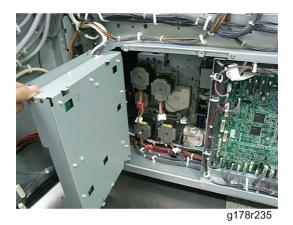
4. The picture above shows that the IOB 1 bracket is open.
