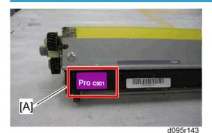
Check that the "Pro C901" decal is attached to the cleaning unit. The drum cleaning unit with the "Pro C901" decal can be used for the Pro C901 and Pro C901S models. Never use a drum cleaning unit for predecessor models. If the wrong type of drum cleaning unit is installed, image problems may occur due to insufficient drum cleaning.
