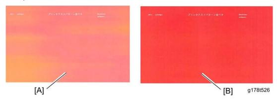
Here is a sample image if an abnormal image occurs on an output due to the incomplete connection of CN412.
