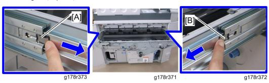
3. Release the hooks [A] [B] at the left and right rails of the ITB unit drawer, and then pull the ITB unit drawer out a little bit.
