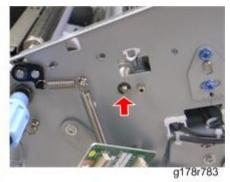
6. Pull out the shift roller unit shaft [E] toward the rear side ( $\mathbb{C} \times 1$ : front, spring  $\times 1$ )
