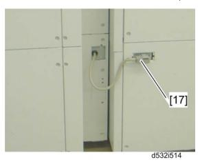
26. Attach I/F connector [17] of the 2nd LCT to the 1st LCT.
