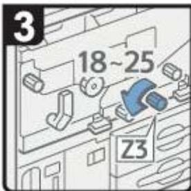
Rotate the knob Z3 counterclockwise, 18 to 25 times.
