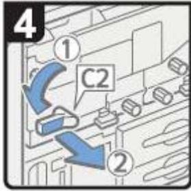
Turn the C2 lever and pull out the fusing unit drawer.
