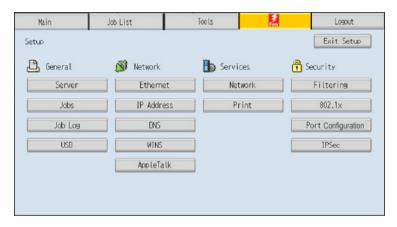
If your network uses DHCP, the Pro C900 acquires the IP address automatically. Otherwise, enter the Pro C900 address.
