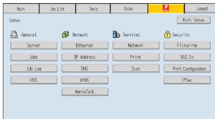
If your network uses DHCP, the Pro C900s acquires the IP address automatically. Otherwise, enter the Pro C900s address.
