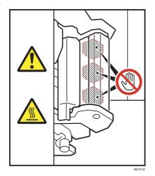
Do not touch the parts a label indicates. The inside of the Booklet Finisher SR5020 could be very hot. Caution should be taken when removing misfed paper.
