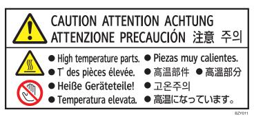
High temperature parts. Do not touch the parts which a label is put on. Otherwise, an injury might occur. 4
