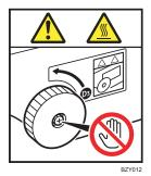
The screw hole in the center of the knob gets very hot. Do not touch this area. Doing so could result in burns.
