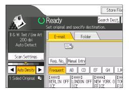
Using the number keys, enter the five-digit registration number assigned to the required destination.
