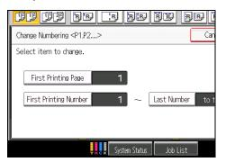
3. Press [First Printing Number], enter the number of page from which to start numbering with the number keys, and then press [#].
