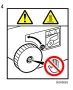
The screw hole in the centre of the knob gets very hot. Do not touch this area. Doing so could result in burns.
