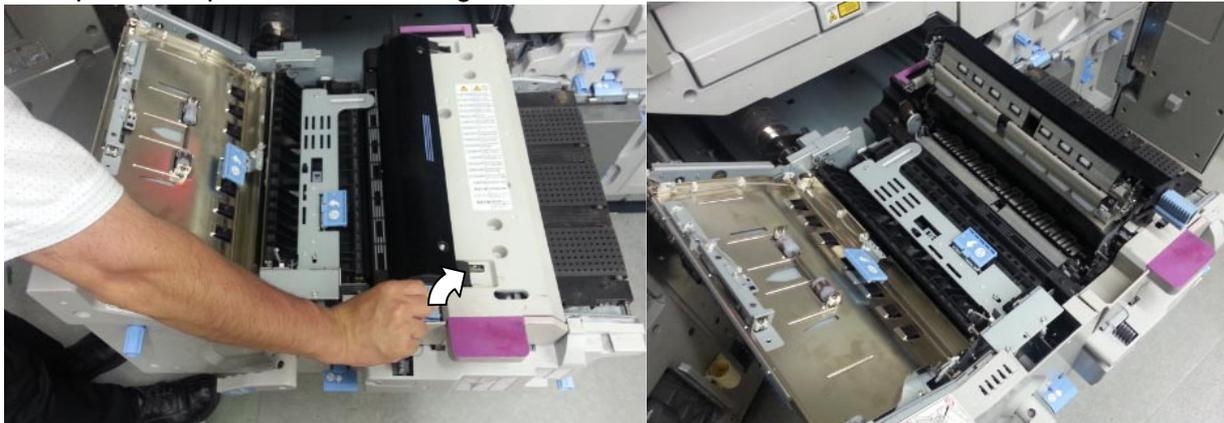
3. Place a sheet of paper to prevent damage to the guide plate.
