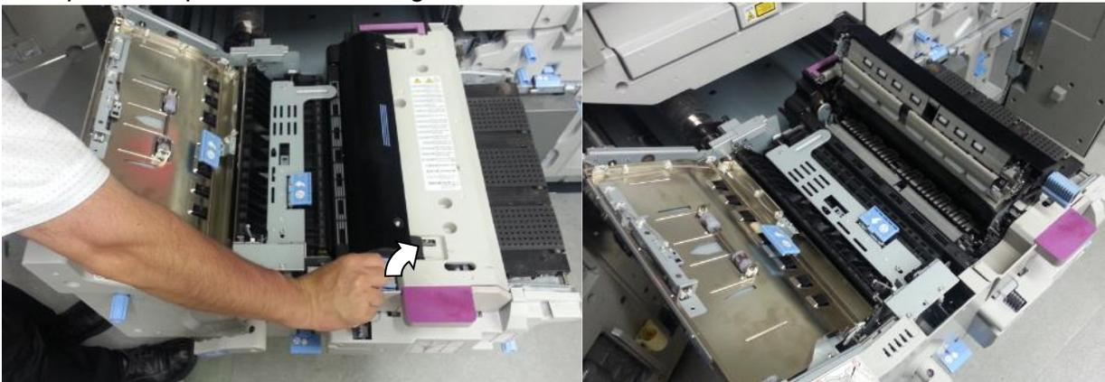
3. Place a sheet of paper to prevent damages to the guide plate.
