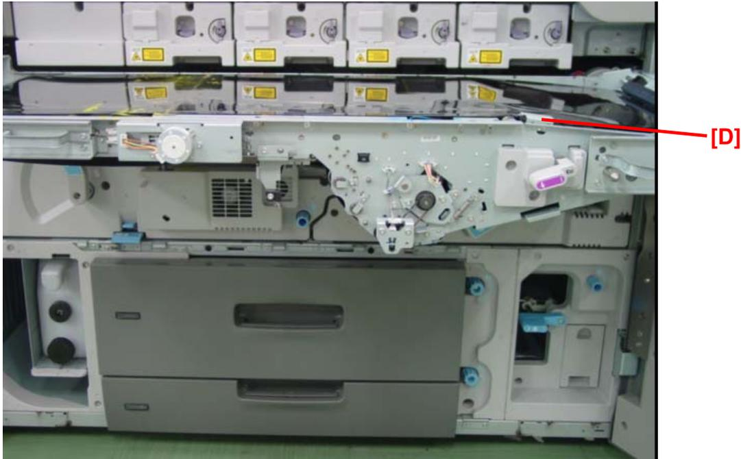
5. Remove the sensor bracket [D] (Screw x1).
