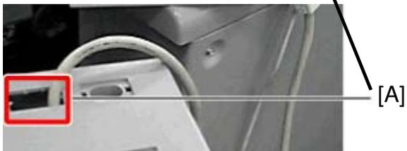
5. Route the key card cable through the hole [A] on the top of the controller box
