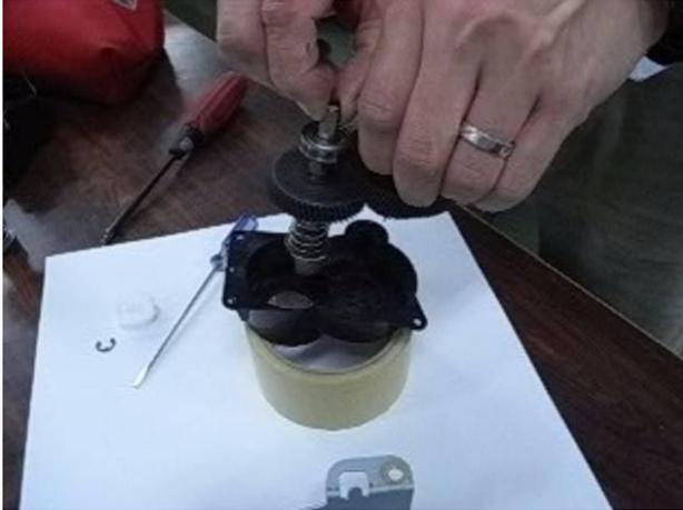
14. Take grease from the gear installed in the old shaft assembly and apply it to the gear installed in the new shaft assembly.
