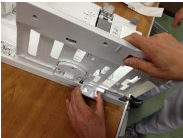
5. Attach the side fences to the tray by hooking the slit [A] on the hinge [B].
