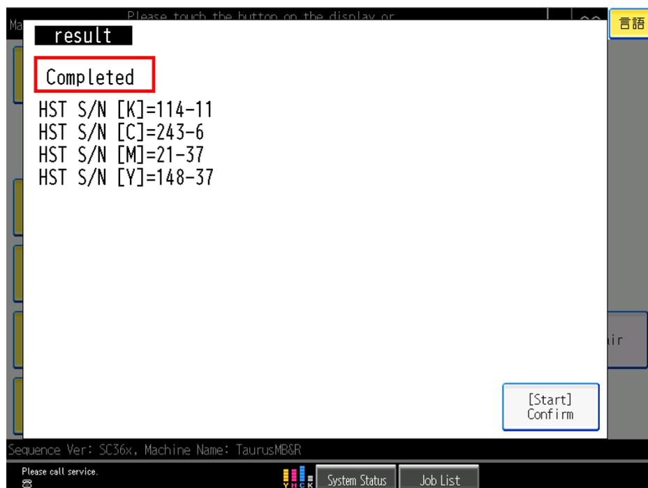
8. If the firmware is not affected by a bug, “Completed” will appear on the display. Go to page 9 of this bulletin.
