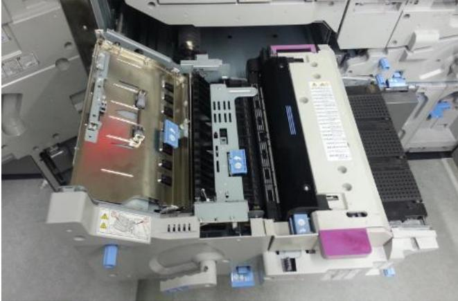
2. Open the top cover of the fusing unit.
