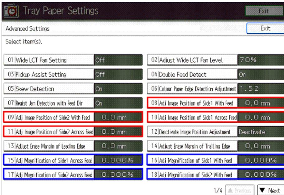
First, adjust the image to the best position\* by making adjustments in the menu items #08-11 indicated with the red boxes in the above diagram. Then, adjust the image size in #15-18 indicated with the blue boxes.
