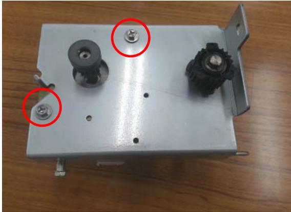
6. Remove the motor. (screw x2)
