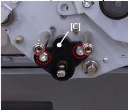
16. Replace the bracket on the rear side with D0743814 / D0743809.
