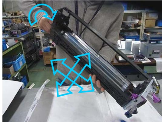
8. Again, hold the development unit as shown in the photos below and shake the unit vertically and horizontally.
