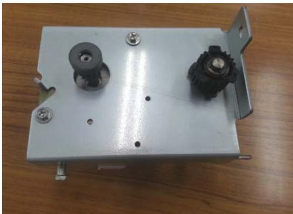
5. Detach the motor bracket from the punch unit.
