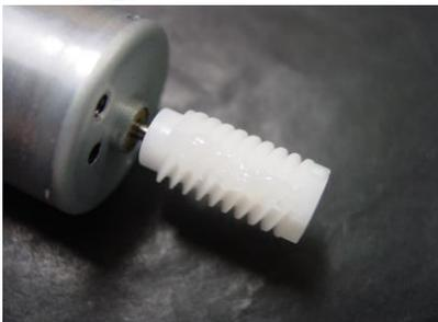
9. Reinstall the motor and gear to complete the procedure.
