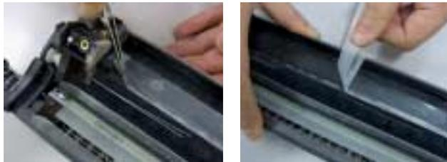
**3-1. Remove the sheet mylar from the frame and clean the surface with solvent so that adhesives do not remain.**
