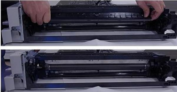
2. Tilt the unit 90 degrees so that the left side (viewed from the front) faces the bottom, then rotate the dev roller in the direction indicated with the arrow (counterclockwise viewed from rear) until the loose developer on the roller surface is cleaned off.
