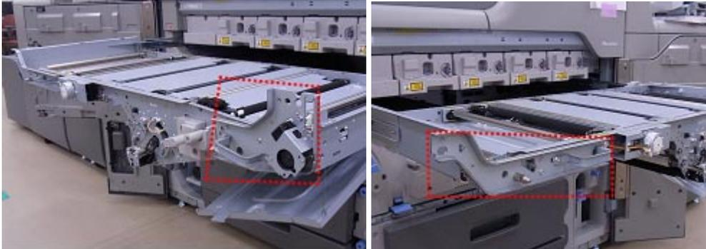
3. Lift up the YMC image transfer rollers by rotating the gears.
