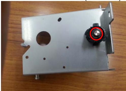
7. Remove the gear. (E-type retaining ring x1)
