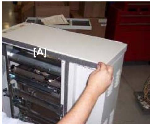
3.3. Attach the spacer cushion [A] (SPACER CUSHION: B8321371) to the top edge of the punch unit.
