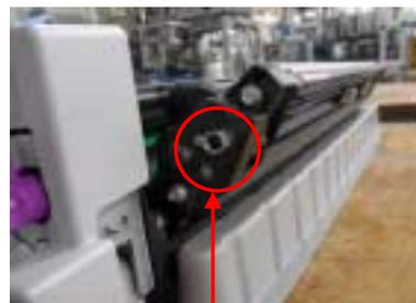
Hollow shaft on the drum cleaning unit
