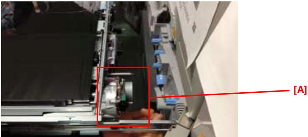
1. Pull out the ITB unit to the second position according to the service manual in the section:
