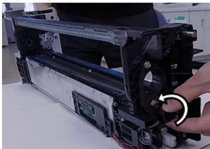
3. Insert the cleaning tool into the doctor gap from the corner without the angled tab. The tab scrapes off the toner/dust adhered to the doctor blade as you slide the tool across the doctor gap.
