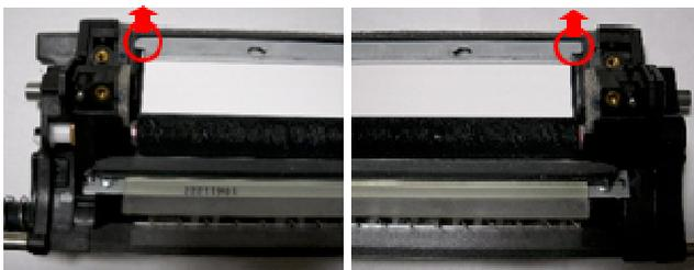
**1-3. Lift up the areas marked with red circles to release the pressure, and then, remove the lubricant bar.**
