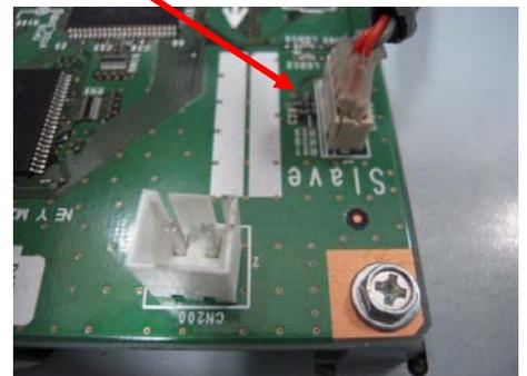
5. Connect the debug cables to each of the connectors on the BCU board.
