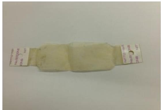
**NOTE:** It is recommended to replace the web (M0774288) after each polish; 1 web per 1 fusing belt.
