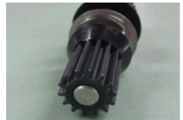
**How to identify the marking on the Coupling Gear on the Development Unit**
