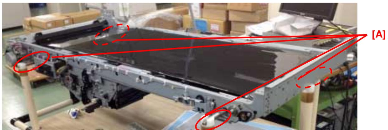
If possible, remove the entire ITB unit from the mainframe because it will be easier to perform the procedure. In this case, the unit should be supported by its shafts [A].
