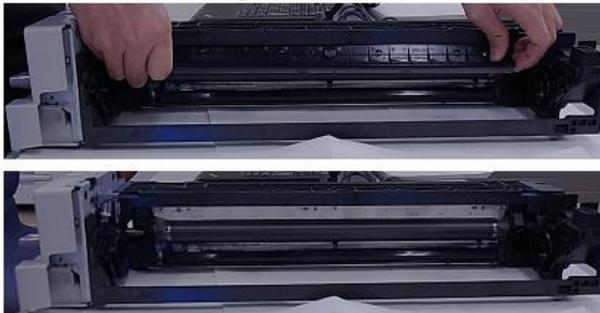
2. Tilt the unit 90 degrees so that the left side (viewed from front) faces the bottom, and then, rotate the dev roller in the direction indicated with the arrow (counterclockwise viewed from rear) until the loose developer on the roller surface is cleaned.
