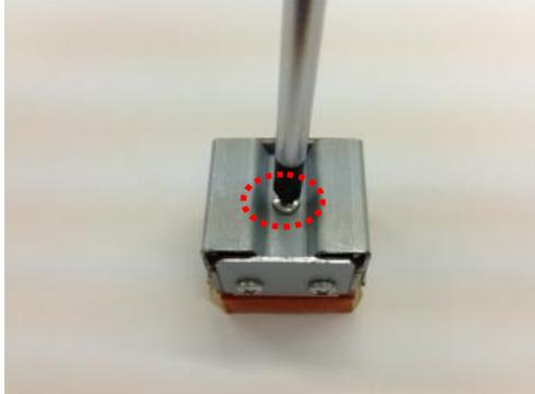
2. Remove the metal plate [B] from the tool [A].
