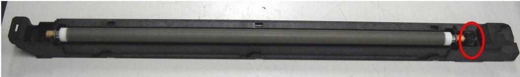
1. Remove the drum charge unit from the PCDU and locate the gear.
