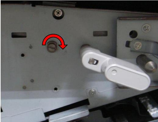
**If the shaft rotates smoothly:** The harness from the motor could be damaged or not connected properly. Check the harness.
