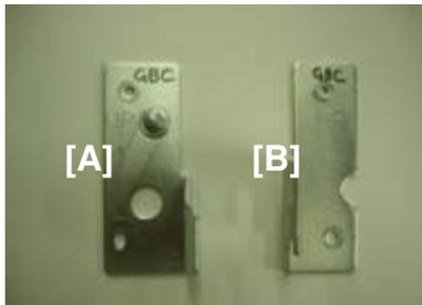
**Step 2. Removing the guide plate supplied with the GBC Stream Punch**
