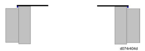
4. The flanges must be set so that both edges of the fusing belt rim overlap the collar of the flanges.
