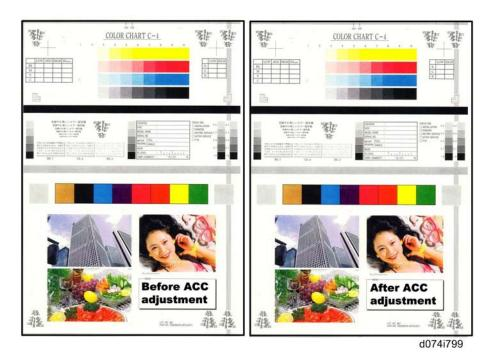
13. Compare the results of the first copy marked "Before ACC adjustment" and the and the second copy marked "After ACC adjustment".
