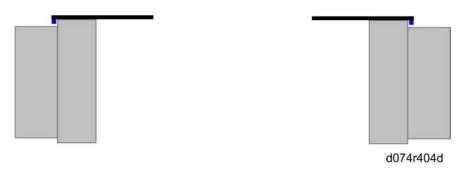
4. The flanges must be set so that both edges of the fusing belt rim overlap the collar of the flanges.
