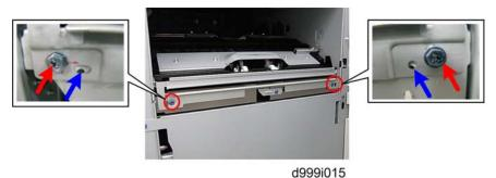
4. Attach the guide plate with the screws removed in Step 2.
