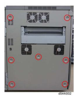
3. Remove the left cover of the main machine (  $\slash\hspace{-0.4em}P$  x7).
