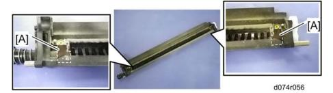
1. Remove the side seals [A] on the cleaning unit.
