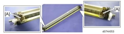
1. Remove the side seals [A] on the lubrication unit.
