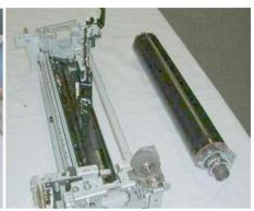
29. Lift and remove the pressure roller, and then place it on a flat clean surface.
