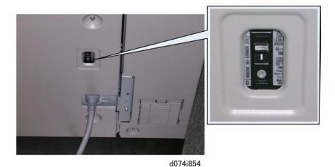
The breaker switch is at the bottom corner of the rear right side of the machine. The optional ring binder also has a breaker switch.
