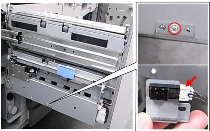
2. Disconnect the sensor bracket and remove the sensor ( ₱x1,₺ x1, x3).
