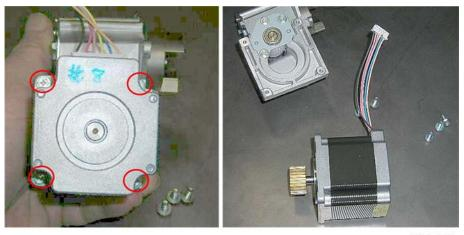
4. Remove the motor from the drive bracket (  $\slash\hspace{-0.4em}P$  x4).
